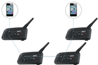
Four V4 pairing diagrams
