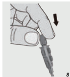
8. Glide the foam bonnet on the microphone end.
